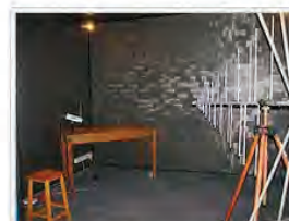
Anechoic RF chamber used for EMC testing (radiated emissions and immunity). The furniture has to be made of wood or plastic, not metal.
