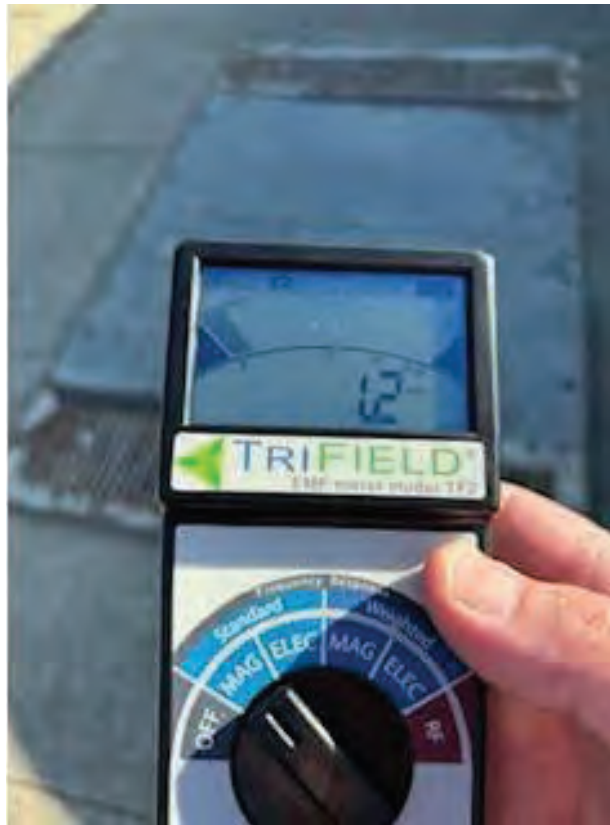
An underground transformer at 29 Wildwood- it is possible, and it puts out a lot less EMF than the transformer on the next page!
