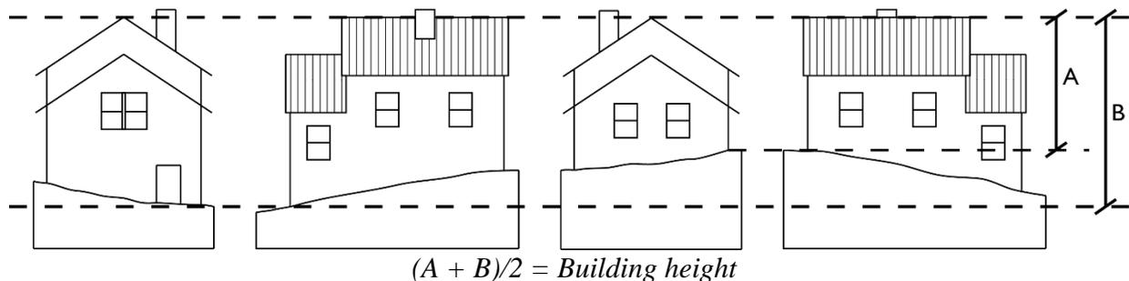
*Building height of an accessory dwelling unit* is measured from the average level of the highest and lowest point of that portion of the ground covered by the footprint of the *accessory dwelling unit* to the highest point of the roof edge, mechanical equipment, or parapet wall. *Building height of an accessory dwelling unit* is not measured to the highest point of a chimney or communications antenna.
