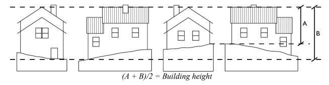
Building height of an accessory dwelling unit is measured from the average level of the highest and lowest point of that portion of the ground covered by the footprint of the accessory dwelling unit to the highest point of the roof edge, mechanical equipment, or parapet wall. Building height of an accessory dwelling unit is not measured to the highest point of a chimney or communications antenna."
